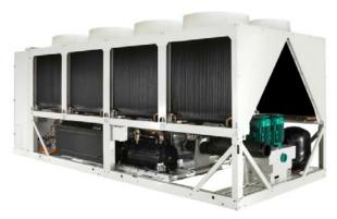
The 2 units use an asynchronous motor speed variation system, a control system based on floating low and high pressure. The key element in this project is that these 2 units have heat recovery systems. Indeed, the heat created during the production of chilled water is reintroduced into the batteries of the complete air treatment system. The whole project represents an investment of about €300 K and benefits from the energy certificates scheme.
